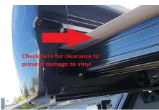
Place a piece of paper with masking tape inside the case below the holes before drilling to reduce debris being trapped inside the awning case which may damage the awning or blow into your eyes next time you set up. Drill the holes using a 5mm drill bit. Ensure the drill chuck does not damage your awning vinyl when drilling, place a piece of cardboard between the drill and vinyl if necessary. With the roof up you can insert the pop rivets from behind to allow the rivet gun easier access.
