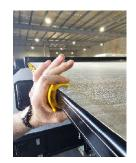
With the anti flap Kit in place you can now add walls feeding from the gap in the centre of the bar out towards each end. NOTE: Seams and tags are on the INSIDE of the shades.
